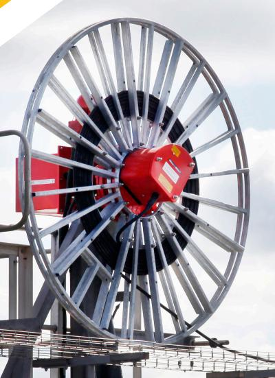
Metreel is one of the leading suppliers of cable reeling systems, typically being utilised for the safe supply of power and controls to cranes, hoists, materials handling plant and travelling machines.
