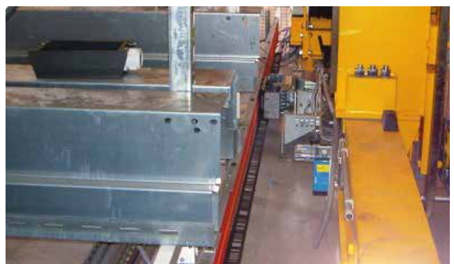
Application of a 10-pole Pro-Ductor system with code rail
