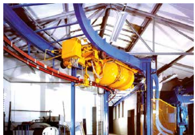
Feed and control of a concrete skipper
