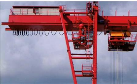
Our festoon systems offer extensive options for the safe and efficient transport of your cables. Thanks to the high quality and reliability, you can use it for situations, both indoors and outdoors.
