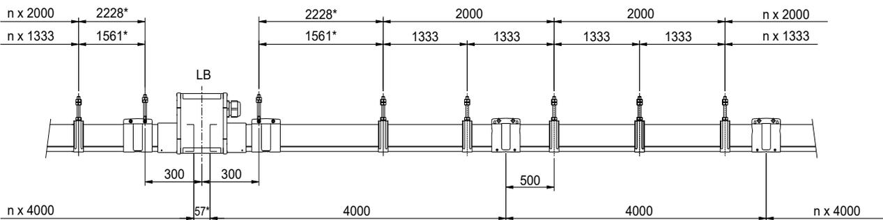
When clamp holder RN-LH is applied: 57 = 0 mm; decrease other dimensions marked with \* by 28 mm
