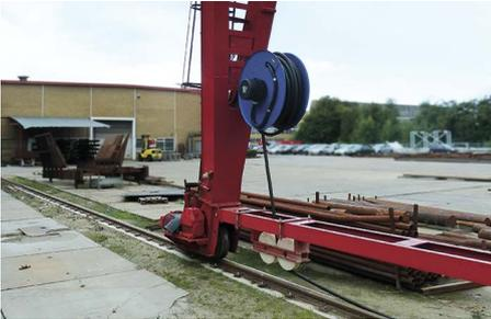
Our cable reels prove their worth daily in numerous applications, indoors as well as outdoors. Reliable power consumption and control for cranes, hoists, internal transport carts, electrical tools etc. We can also supply the correct high-flexible cable to meet your needs!
